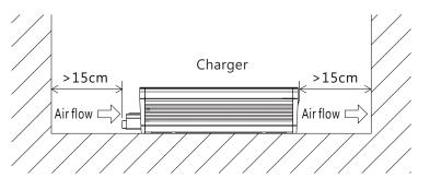
Figure 3-1 set-up recommendation
